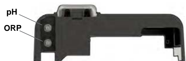
Figure 19. pH/ORP Connection Ports
