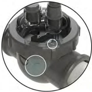
Figure 16. POD Locking Ring Orientation
