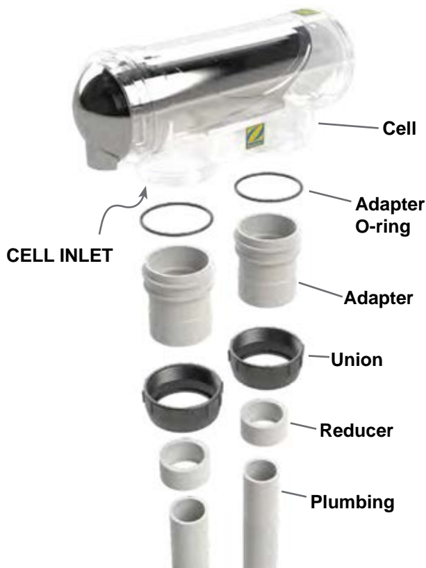
Figure 5. Cell Plumbing Assembly
